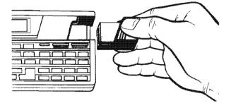
5. Slide the cartridge to the left until it snaps into place.
