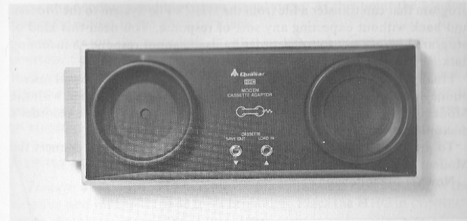
Figure 9-13. Modem with Cassette Interface
