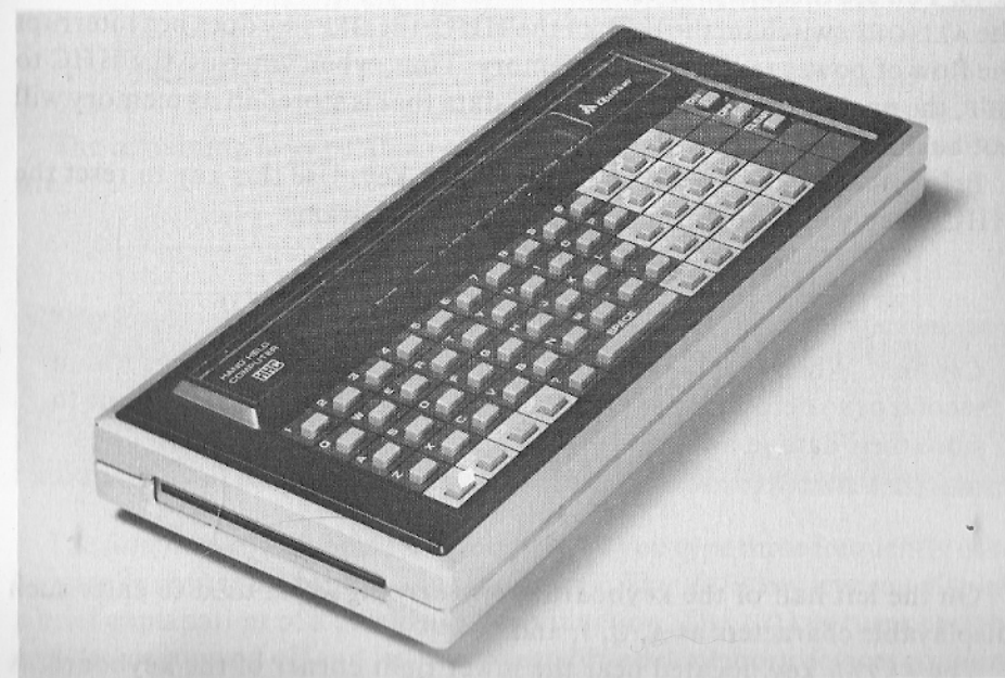
Figure 2-5. Left side of HHC: bus slot
