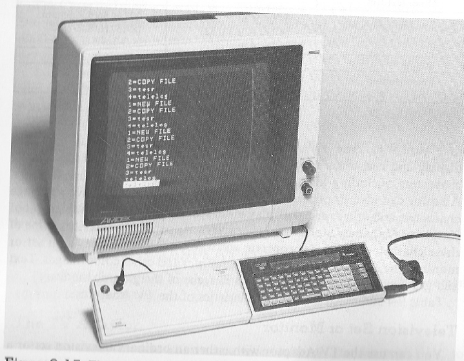
Figure 9-15. The TV Adaptor and HHC with a video monitor
